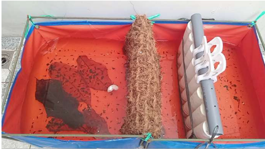
Picture 8. Half of the Mosquito Dunk® settles in the imitation drainage system shortly after application
