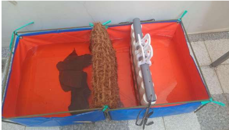
Picture 2. Real-life prototype of MosqBlock Concogtion placed in an imitation drainage, with dry leaves to imitate fallen debris.
