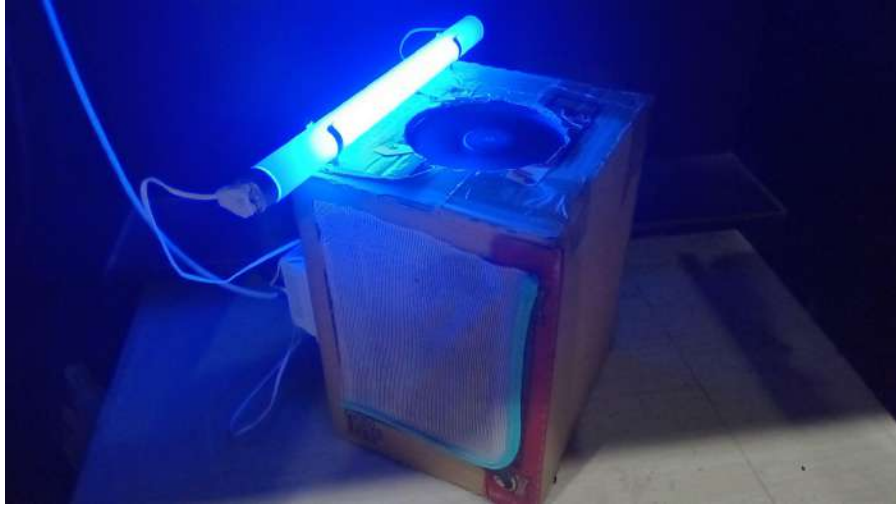
Picture 3. Mosquito trap placed in a dark spot, under a table, to attract mosquitoes and keep track of them.
